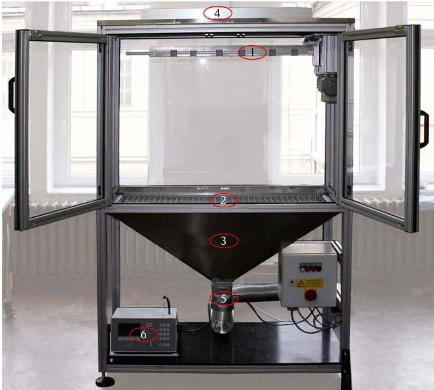
Fig. 19: Test unit to determine the particle contamination in the range of 0.3 to 10 \mu\text{m} . 1 support rail for the maps, 2 grating, 3 funnel, 4 superfine filter for air intake, 5 isokinetic sampling probe, 6 light-optical particle measuring device.
