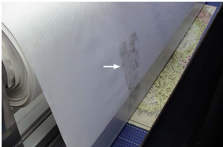
Fig. 12: View of the film with the dirt removed from the surface (arrow).
