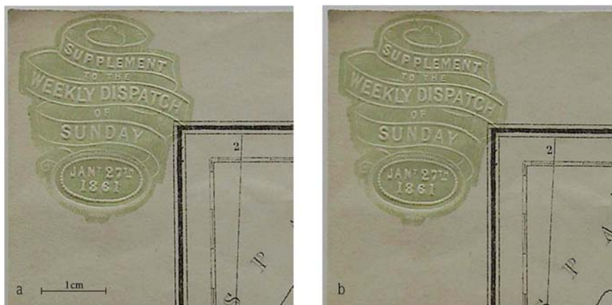
Fig. 17: Embossed stamp from the map no. 547$11133960X before (a) and after (b) being passed through the cleaning machine.
