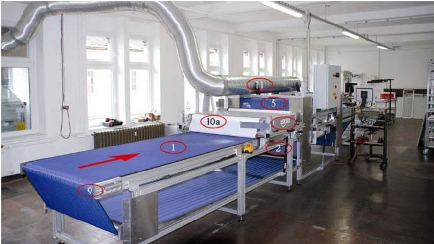
Fig. 8a: Electrostatic cleaning system Gothana : 1 conveyer belt (loading end / cleaning module I), 2 suction device I, 3 cleaning module I, 5 conveyer belt (cleaning module II), 9 synchronized drive unit, 10a electrostatic film infeed (cleaning module I), 11 exhaust unit.
