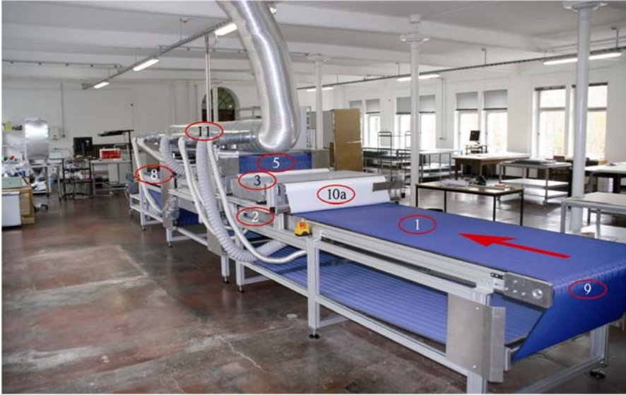
Fig. 8c: Electrostatic cleaning system Gothana : 1 conveyer belt (loading end / cleaning module I), 2 suction device I, 3 cleaning module I, 5 conveyer belt (cleaning module II), 8 conveyer belt (discharge end), 9 synchronized drive unit, 10a electrostatic film infeed (cleaning module I), 11 exhaust unit.
