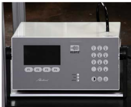
Fig. 20: Light-optical particle measuring device – Klotz Ama LDS 0.3/10.
