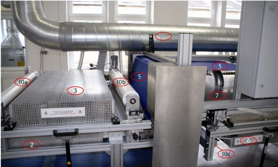
Fig. 8b: Electrostatic cleaning system Gothana , dust removal unit: 2 suction device I, 3 cleaning module I, 5 conveyer belt (cleaning module II), 6 cleaning module II, 7 suction device II, 10a electrostatic film infeed (cleaning module I) 10b winder for spent electrostatic film (cleaning module I), 10c electrostatic film infeed (cleaning module II), 11 exhaust unit.
